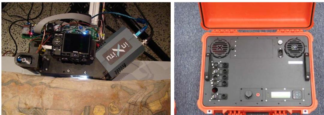
Figure 6. The portable reflection XRD/XRF instrument; Left: Early implementation of the prototype (no cover) positioned for analysis of a red shroud Fayum mummy from the Getty Museum; Right: Portable power unit of the instrument that includes Li-ion batteries, AC adapter, embedded computer, lighting controls, LCD for basic control, and WiFi communication for full remote control using any handheld or laptop computer through html interface
