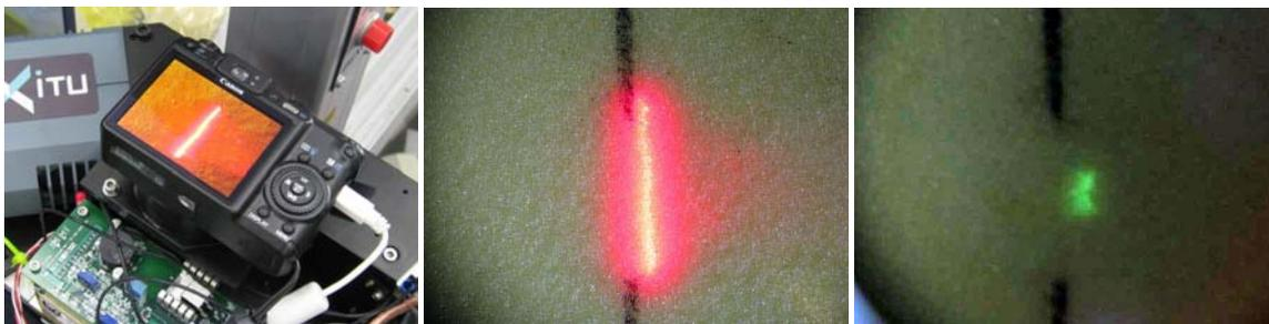
Figure 5. Left: Imaging camera fitted to the instrument. High magnification images collected on the surface of a phosphor screen with the alignment laser (center) and X-ray spot (right).
