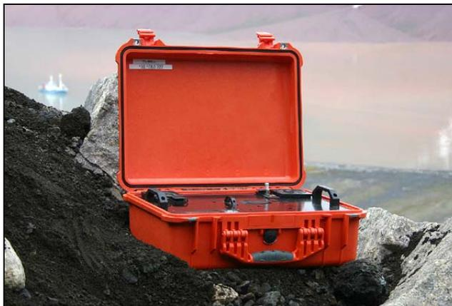
*Figure 1: Portable XRD-XRF instrument Terra developed and marketed by inXitu Inc. Based on a transmission geometry, it requires insertion of crushed materials ( $<150\ \mu\text{m}$  grain size) in a vibrating sample cell<sup>10</sup>*
